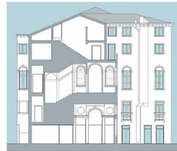
THE OLD FACADE HAS BEEN COVERED IN THE 1700 FROM A STAIRCASE THAT CONNECTS THE TWO BUILDINGS
